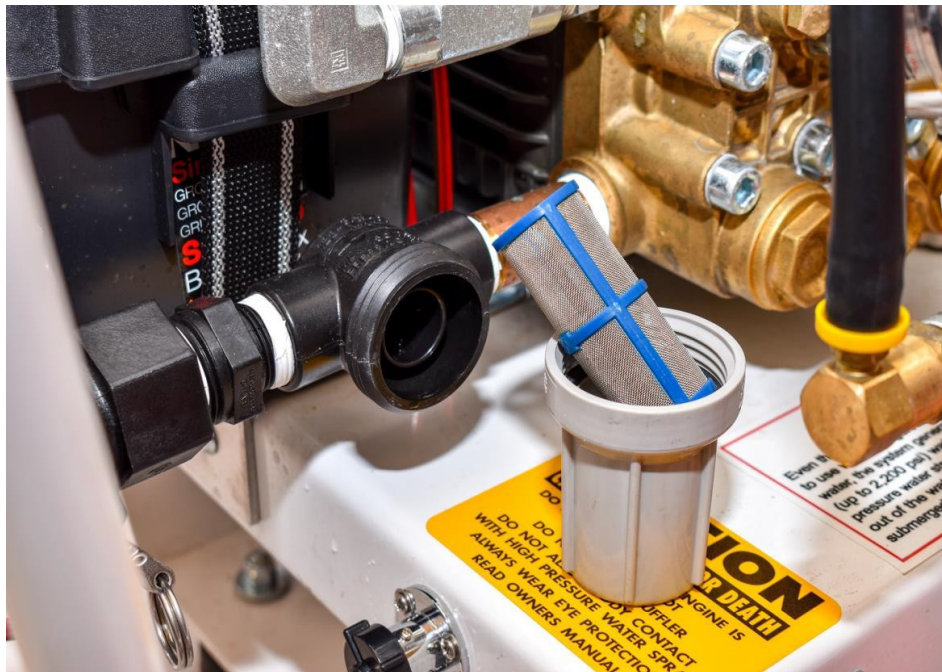
Water Inlet - Figure #1
