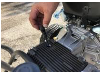
Pump Oil Level - Figure #3
