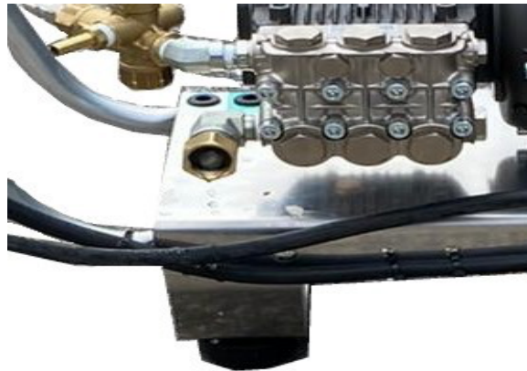
Figure #4 - Connect Garden Hose to Water Inlet
