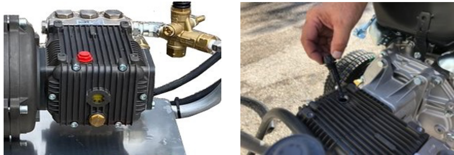
Figure #2 - Pump Oil Level
