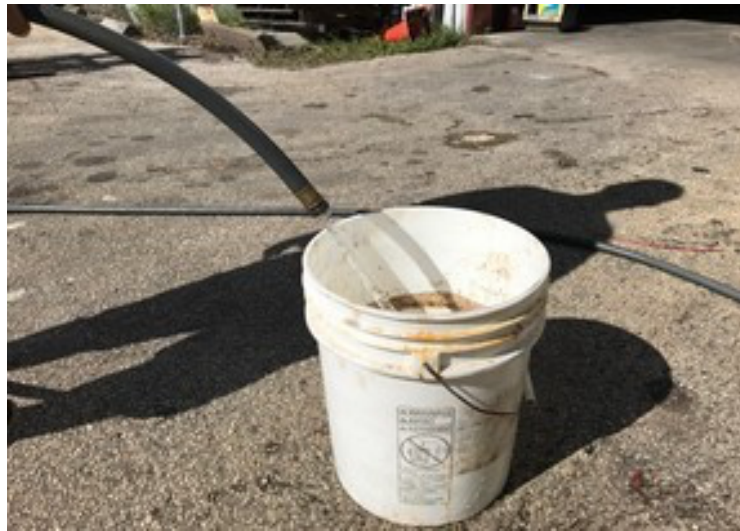
Figure #5 - Fill Up a 5-Gallon Bucket in Less Than One Minute
