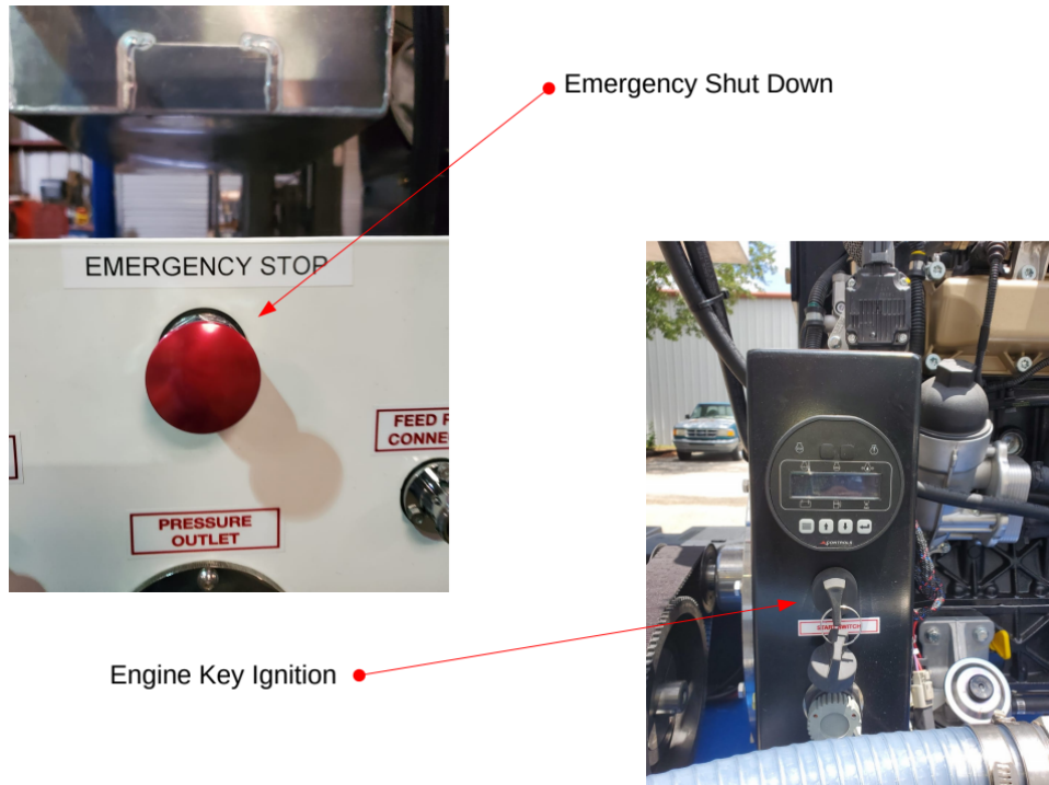
Figure 5.1 – Engine Emergency Shut-Down and Throttle Control
