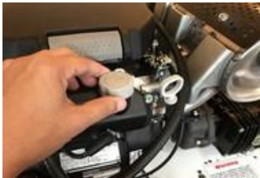
Figure # 5 – Engine Oil Fill Port
