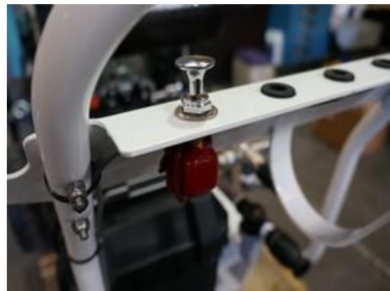
Figure # 12 – Feed Pump On/Off Switch
