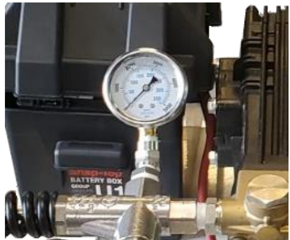
Figure # 20 – Pressure Gauge
